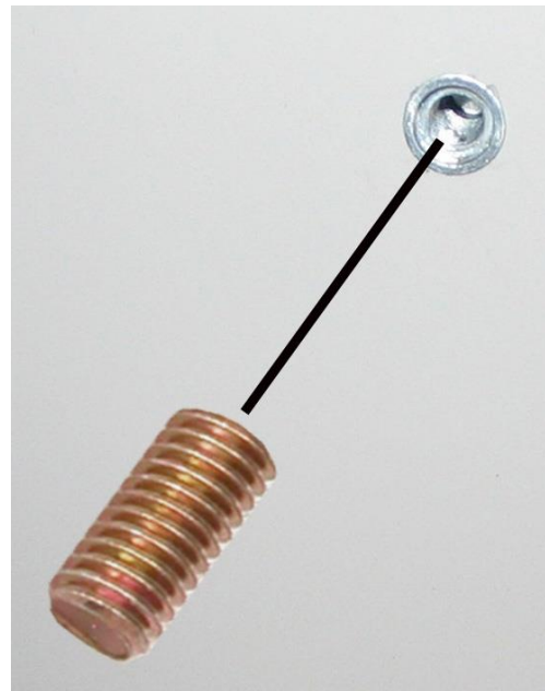
Step 17 screw in studs into threaded inserts
