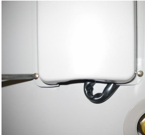
Step 2 remove screws from lower front cover
